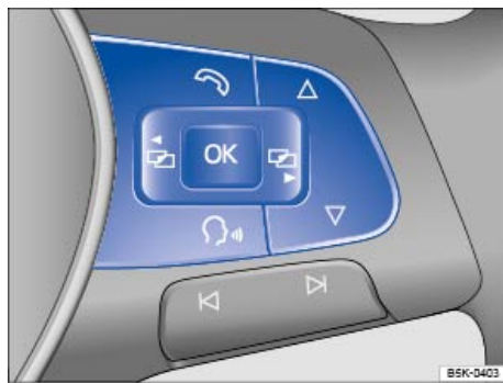
Fig. 14 Right side of the multi-function steering wheel (if equipped): Controls for the menus and information displays in the instrument cluster.
