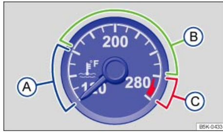
Fig. 169 Engine coolant temperature gauge in the instrument cluster: A Engine cold; B Normal temperature range; C Warning zone.
