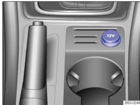
Fig. 124 In the lower center console: 12 Volt socket.
