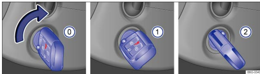
Fig. 127 In the ignition switch: Vehicle key positions.
