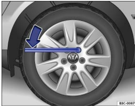
Fig. 191 Changing a wheel: Loosening the wheel bolts.
