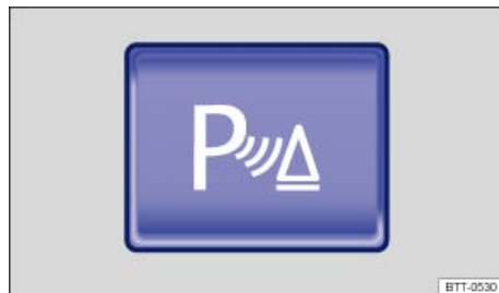
Fig. 150 In the center console: Button to switch the Park Distance Control system on or off.
