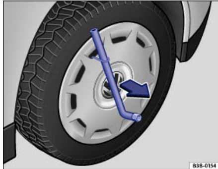
Fig. 190 Pulling the wheel cover off.
