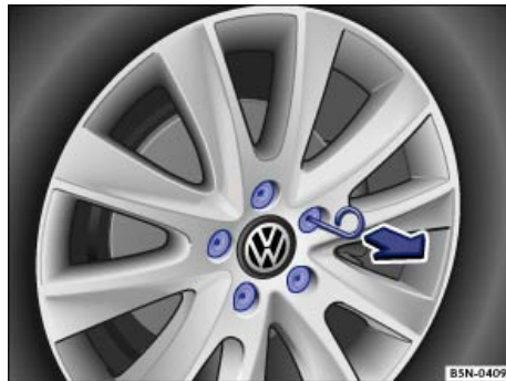
Fig. 189 Pulling cover caps off wheel bolts.
