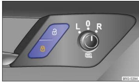
Fig. 23 In the driver and passenger doors: Power locking button.
