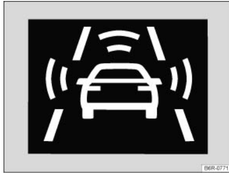
Fig. 154 In the instrument cluster display: Advance warning (symbol displayed in color on an instrument cluster with color display).
