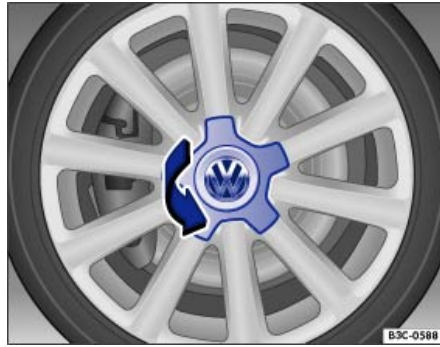
Fig. 188 Twisting the hubcap off.
