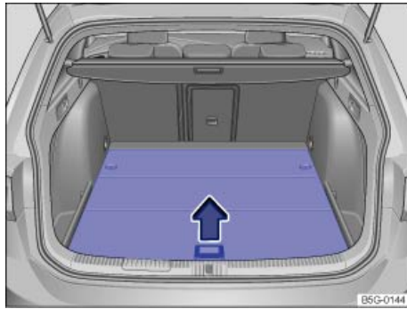
Fig. 185 In the luggage compartment: Opening the luggage compartment floor.
