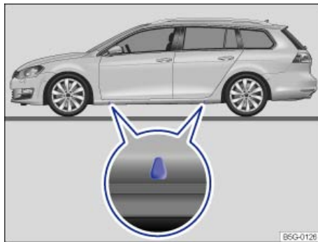
Fig. 192 Lift points for the jack.
