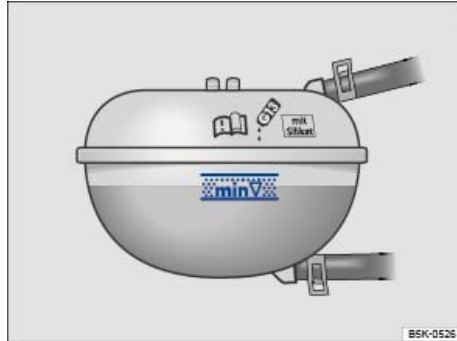
Fig. 170 Coolant expansion tank in the engine compartment.
