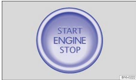
Fig. 128 In the lower center console: Starter button for the Keyless Access system.
