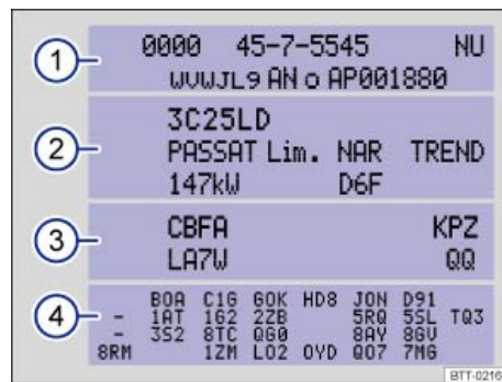
Fig. 16 Vehicle identification label: Shown in the example with engine identification code CBFA 3.
