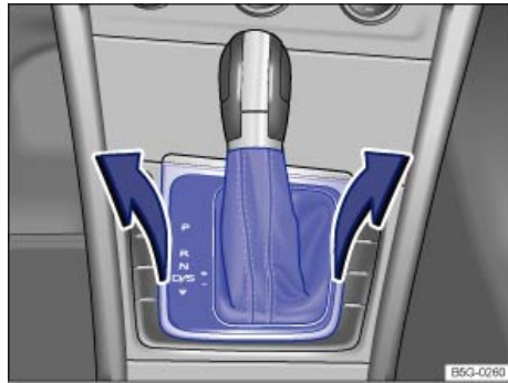
Fig. 182 Removing the selector gate cover.
