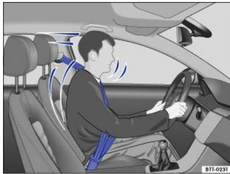
Fig. 53 Belted driver secured by the correctly worn safety belt in the event of a sudden braking maneuver.
