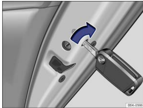
Fig. 179 On the front side of the right rear door: Locking the vehicle with the key bit in the vehicle key.
