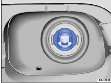
Fig. 162 With open fuel cap: Misfueling guard in the fuel filler neck.
