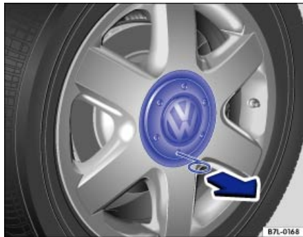
Fig. 187 Pulling the hubcap off.
